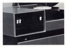
Disc drive 3665 uses a new recording technique to provide 480 million megabytes on-line. The bits/track are doubled and the rotational speed is reduced to 1200 rpm, thus maintaining 312 kbits transfer rate compatibility with the System/360. The 3665 consists of a 661 controller with a 665 (double density) adapter and from one to eight 665 drives plus spare. Unit accepts standard 2316 disc pack. Memorex Corp., San Tomas at Central Expressway, Santa Clara, CA 95052.
