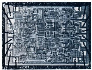
IC contains 4 input preamps, an output amplifier and decode/control circuitry in 16-lead hermetically-sealed DIP.
