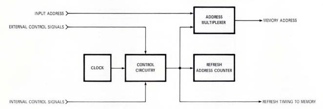
Fig. 3-Block diagram illustrates basic arrangement for refreshing a dynamic memory.
