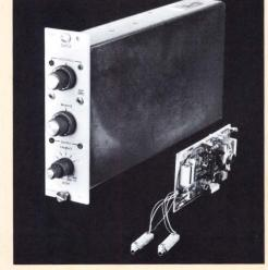
gage excitation. It also has two-level positive and negative calibration, a provision for double shunt calibration.
