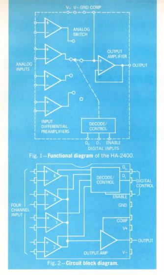
"Instrument on a chip" is a step closer to reality with a new concept in ICs introduced by Harris Semiconductor. Actually, instruments (plural) would be more accurate because this DIP building block (called the HA-2400 PRAM) can be used to construct a variety of circuits. The significance of this development is not in the complexity or in the amount of circuitry packaged on a chip, but in the versatility provided by the packaging concept and design.
