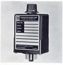
Solid-state time delays, TSR and TSS, are of the fixed and adjustable type for industrial and commercial applications. The TSR has a dpdt, 10A output and the TSS has an spst, 2A output. Both are available for 12 to 230V inputs and time ranges from 0.1 to 480 sec. Syracuse Electronics Corp., Box 566, Syracuse, NY 13201. 219
