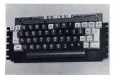
**Keyboard,** Model MK-29, offers L-shaped keys and deep-dished "home position" keys for added operational ease and efficiency. Standard features include 51 keys (MK-29/2011), encoded and function keys, two-key rollover, error and data lockout and DTL/TTL compatibility. The keyboards are insensivive to RFI and electrostatics. Typical power requirements are 5V, 180 mA. Data Electronics Corp., 12 Cambridge St., Burlington, MA 01803.
