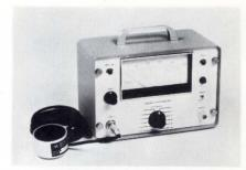
Portable photometer priced at \$295 each is available with a selection of four different probes with sensitivity to 0.0002 footcandles. Features of the Model 3100 include sensitivity from 0.001 to 10,000 footcandles, 5% full-scale accuracy, 3% linearity and a recorder output of 1V to 1 mA. Vactec, Inc., 2423 Northline Industrial Blvd., Maryland, MO 63043.
