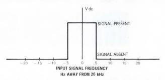
Fig. 4- **Output** of the threshold detector (**Fig. 1**) set for large S/N ratio operation.
