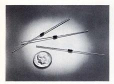
Silicon voltage regulator zeners with low dynamic impedance and low bias current requirements are presently being produced with a nominal voltage of 30 to 120V for 1, 3 and 5W applications. The zeners exceed military and aerospace specifications, and are of noncavity monolithic construction with a fused metal hermetic seal. Semtech Corp., 652 Mitchell Rd., Newbury Park, CA 91320.
