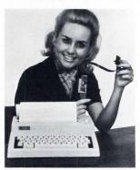
Low noise level and 300 words a minute are the major advantages of NCR's new 260 data terminal. By eliminating the conventional ink-and-impact printout concept, NCR has made a significant reduction in ambient noise that should be welcome in computer rooms.
