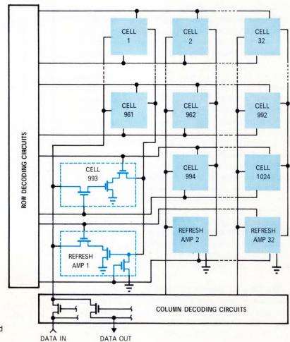
Fig. 2—Basic cell arranged in a matrix form.
