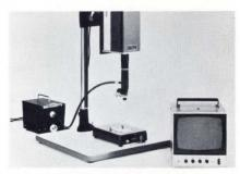
Television-microscope system, Model MV 9000, is a fully coordinated CCTV system for microscopic examination up to 600 power. It includes a high-resolution camera, a solid-state monitor, complete optical system, adjustable camera platform and a fiber-optic illumination system. Circon Corp., Santa Barbara Airport, Goleta, CA 93017.
