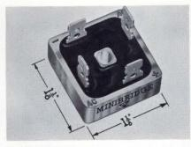
Silicon bridge rectifiers, called "Minibridges," are approximately 1.125 inch² by 7/16 inch high with 0.193-inch-diam centers for convenient mounting to a heat sink. Rectifiers feature beam lead construction. Universal 3-way terminals make wiring and mounting easier. Typical of these rectifiers is the PA05 rated at 8A and 50 PIV. Electronic Devices, Inc. 21 Gray Oaks Ave., Yonkers, NY 10710.
