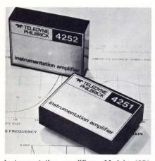
Instrumentation amplifiers, Models 4251 and 4252, are gain programmable over the 1 to 1000 range using one resistor. Other specifications include 2  $\mu$ V/°C input offset voltage drift, <1 nA/°C bias current drift and 30 M $\Omega$  common-mode input impedance. Price in 100 quantities is \$62 each. Teledyne Philbrick, Allied Drive at Rte. 128, Dedham, MA 02026.
