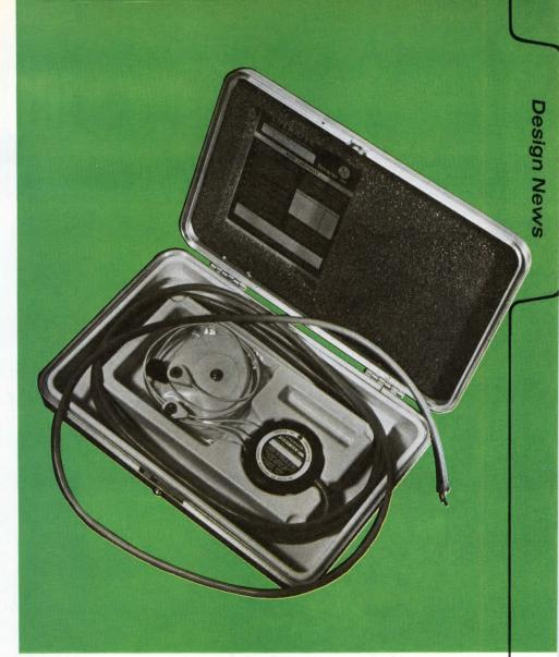
**The "Lifewafer"** is connected to its battery power by biased reed switches which are controlled by magnets mounted inside the case. The reed switches close to energize the unit only when it is removed from the case.
