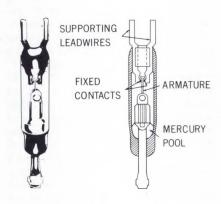
Fig. 1-Low-mass, "T"-shaped pivoted armature moving on a mercury lubricated bearing replaces the conventional stiff spring element in the new HGQM relay.
