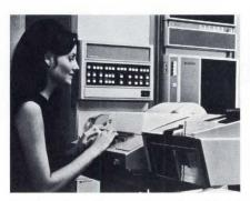
Disc-based small computer system, Model 2120A, combines the Model 2100A computer and Model 7900A moving-head disc with sophisticated software, including extended disc file management capability. Storage capacity is further increased with the addition of the Model 2883A disc drive. Hewlett-Packard Co., 1601 California Ave., Palo Alto, CA 94304.
