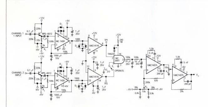
Fig. 5-Phasemeter schematic.
