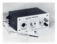
Electronic thermometer features platinum sensing element, no adjustments and fully interchangeable factory-calibrated sensors and electronics. Output is 10 mV/° for use with digital voltmeters, recorders and loggers. Temperature range is -60 to 200°C with ±0.05°C repeatability. Prices for the Model 911 start at \$195 each (including sensor). Stow Laboratories, Inc., 110 Kane Industrial Dr., Hudson, MA 01749.
