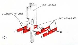
Fig. 1-Side view (A) shows the binary encoded switch (Pat. No. 3472973) and part locations. When the switch is pushed, the pair of contacts on the end will close if the notch is cammed.
