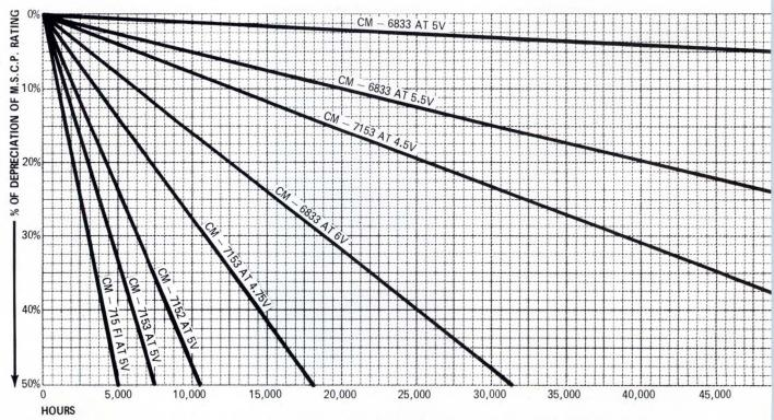
PERCENT OF MEAN SPHERICAL CANDLE POWER DEPRECIATION VS ELAPSED TIME IN HOURS
