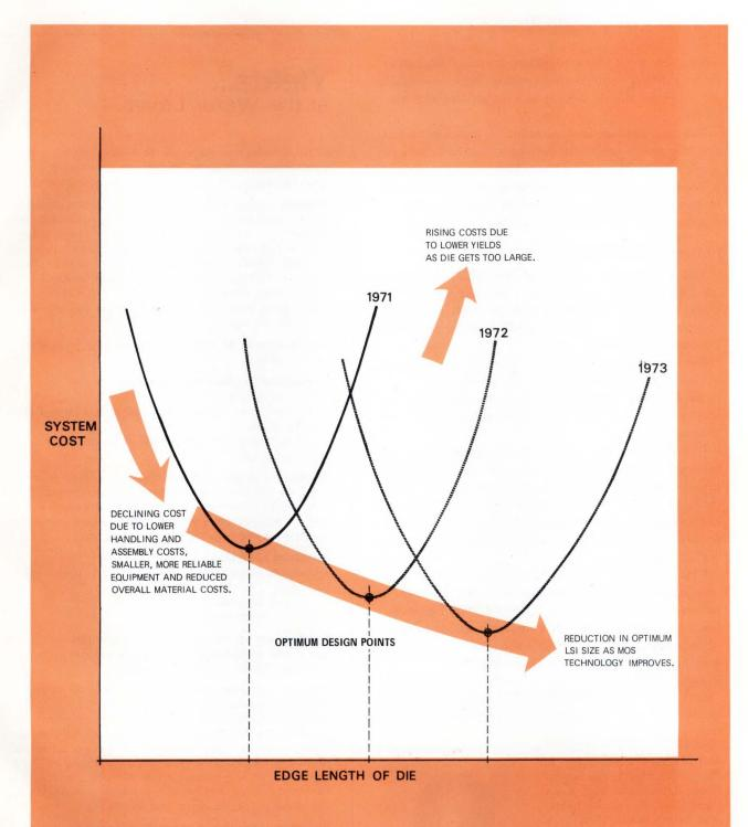
Fig. 3—**Optimum chip size** depends on cost per function. Cost per function depends not only on yield, but also on the handling and assembly costs of the good chips. Increasing the chip size can decrease the handling and as-
