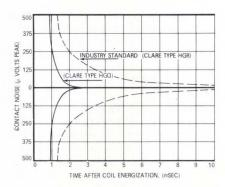
Fig. 2-Contact noise settling to 5  $\mu V$ in 2 msec represents a significant improvement in electromechanical relays.
