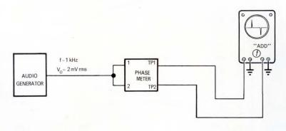
Fig. 6-Test setup matching channel duty cycles.
