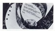
Dual power driver MCH 2890 permits driving of high-current loads directly from logic level devices. This new device translates logic voltage levels to high power outputs. Inputs can be DTL or TTL and loads can be either resistive or inductive. Applications requiring high current pulses that are digitally controlled can now be interfaced with a single package. Motorola Semiconductor Products Inc., Box 20912, Phoenix, AZ 85036.
