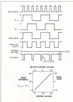
Fig. 2—**Timing diagrams** (upper) and phase-detector characteristics (lower) for the digital PLL.
