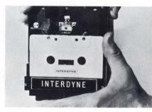
**Cassette tape drive** IC/2500 features a single servo-controlled capstan motor and a pair of individual reel motors for precise tape velocity and tension control. Recording rates are either up to 9600 bps synchronously or from one character at a time up to 30 cps incrementally. Available are a single-gap-head write/read unit for \$995 and a dual-gap-head read-after-write configuration for \$1200. Interdyne, 14761 Califa St., Van Nuys, CA 91401.
