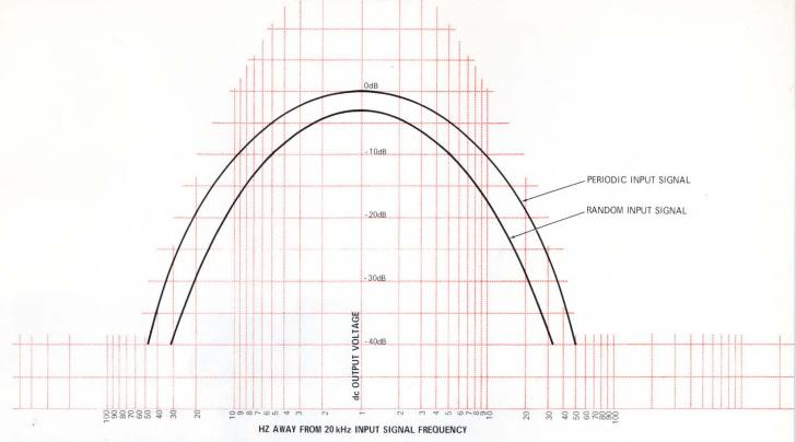
Fig. 3—**Measured output voltage** of the peak-to-peak detector vs input frequency for both random and periodic input signals.
