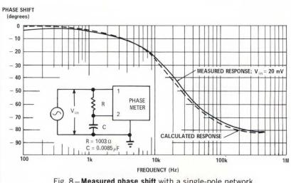
Fig. 8-Measured phase shift with a single-pole network.
