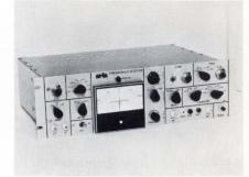
Phase sensitive detector features a digitally derived square-wave reference oscillator output with a linear phase adjustment control. Model ESE3000 has its oscillator and amplifier-detector units completely decoupled and isolated from chassis ground. Frequency range is 10 Hz to 10 kHz with 100 k $\Omega$ /50 pF input impedance. Price each is \$2660. Advanced Research Instrument Systems, Inc., 6500 Tracor Lane, Austin, TX 78721.
