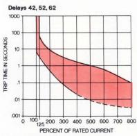
Delays 40, 41 and 42 are for use in 400 Hz systems; delays 50, 51 and 52 are for use in DC systems; and delays 60, 61 and 62 are for use in 60 Hz systems.
