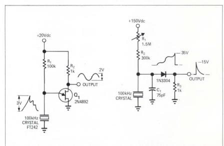
Fig. 1—**Crystal-controlled** relaxation oscillator is similar to RC oscillator except that a crystal replaces the capacitor.
