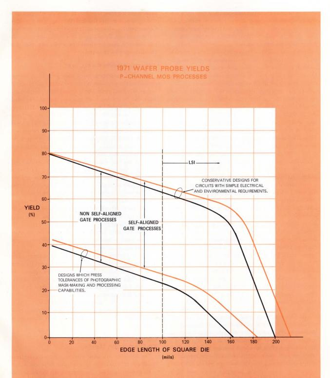
Fig. 2-Chip size vs yield is shown for both a loosely-packed and a densely-packed complex MOS circuit. Maximum yields are 80% and 40%, respectively. Yield
