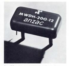
Amplifier, Model MWDH-20G-12, features 20 dB gain (at 10 MHz) and low intermodulation distortion in a plug-in package. Unit operates from 500 kHz to 100 MHz with a frequency response that is flat to 0.5 dB. Typical noise figure is 4.5 dB at 30 MHz, 5 dB at 60 MHz. Anzac Electronics, Div. of Adams-Russell Co., Inc., 39 Green St., Waltham, MA 02154.
