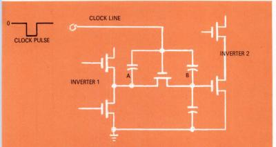
Fig. 1—Improper design always causes low yield. If the capacitive voltage divider for the MOS clocked inverters is not designed properly from a topological standpoint, marginal performance will result. For example, when the clock line goes negative, a negative charge is added to nodes A and B; when the clock line goes positive, a positive charge is added. As clock amplitudes vary, the added or subtracted charge can cause the logical "1" values to become marginal.
