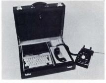
"Data recording and transmission terminal in a briefcase", Model 2002, has full alphanumeric capability, a strip printer and (an option) provides two way communication with EDP center. A cassette recorder, the communications module and a rapid recharger for the nickel cadmium battery are fitted into the briefcase. Both recorder and keyboard can be removed for desk-top operation. MSI Data Corp., 1381 Fischer Ave., Costa Mesa, CA 92627. 258
