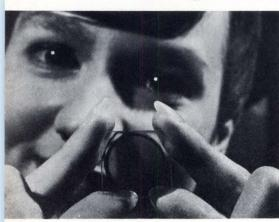
One square inch of a ceramic material, developed by Honeywell Ceramics Center in Golden Valley, Minn., conceivably could hold a 2-million-bit computer memory. This 0.005-inch-thick chip could also be a picture tube for a miniature color TV.
