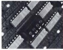
Logic status indicator LL-4D provides four bits of logic status in a DIP. Light-emitting diodes give visible indications, low profile, long life and high reliability. Inputs are TTL/DTL compatible, and each input represents one unit load. In quantities of 1000, the price is \$6.97 each. Unique Devices Co., Box 70, Bountiful, UT 84010.
