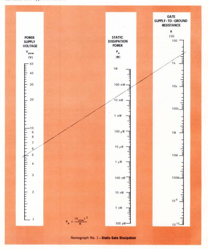
A straight line drawn between the first two values (on the outside scales) intersects the center power scale at 70 mW, which agrees with the value shown in the
