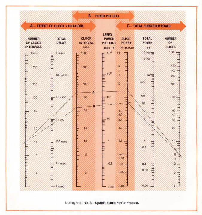
As can be seen from this nomograph, it really pays to keep the signal swing down if you want speed without using inordinate amounts of power.
