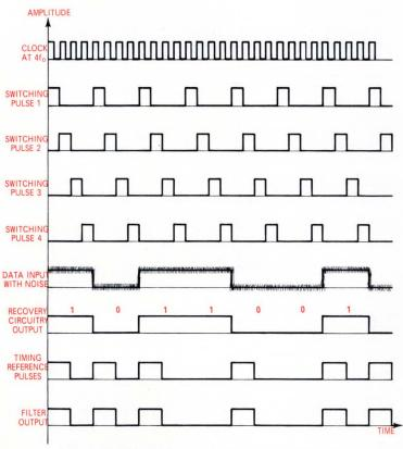
Fig. 2-Waveforms illustrate timing relationship of synchronous and in-phase signals (input and local clock) generated by the system in Fig. 1.
