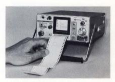
Portable TDR, Model 1501, has a plug-in recorder that permits high resolution recordings at the touch of a button. Its X-Y output is suitable for most oscilloscopes. Step pulse risetime is 1.3 nsec and amplitude is 1V on battery and 10V on ac power. Price is \$1900. Tektronix, Inc., Box 500, Beaverton, OR 97005.
