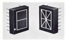
IC-compatible incandescent 5V readout modules provide 7000 fl brightness. The Dip 1050-Digital is a 7-segment device which mounts on a 0.300 inch, 14-pin dual in-line socket. The Dip 1050A-Alphanumeric is a 16-segment device which mounts on a standard 0.600 inch, 24-pin dual in-line socket. Pinlites Div., REFAC Technology Development Corp., 1275 Bloomfield Ave., Fairfield, N J 07006.
