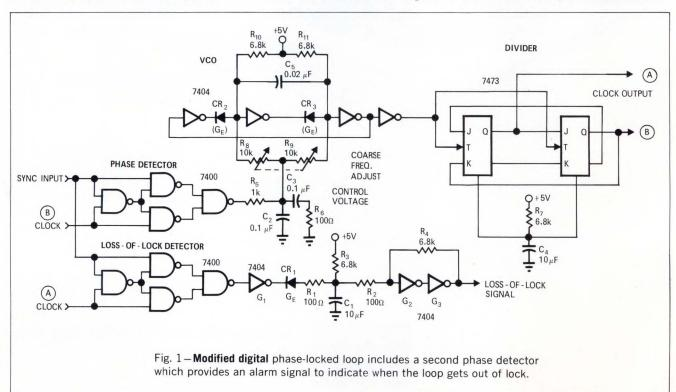
tween the two signals varies  $\pm 90^\circ$  from the normal lock condition, the control voltage swings approximately  $\pm 2V$  from the "zero" value and in a direction which tends to reduce the phase error and bring the loop into lock.
