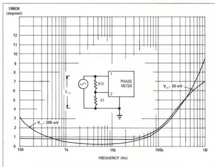
Fig. 7 - Error for 20 dB attenuation between channels.
