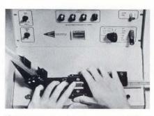
IC test system combines an automatic digital IC tester with a semi-automatic handler. Designed for small- to medium-quantity users, the system uses shipping tubes for both input and output containers. Price is less than \$2000. Electrodata Concepts, Inc., 69 Connecticut Ave., Norwalk, CT 06854.
